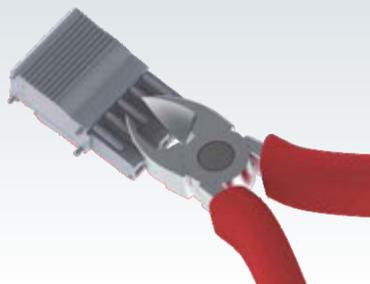
Remove the coding pin from female plug using a cutting tool
