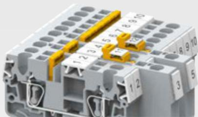
The jumper and marking tag position is aligned across different types of CX series Terminal Blocks. This facilitates shorting and marking adjacent terminals with different functionalities.
