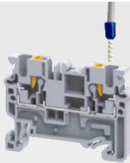
Solid wires and wires with crimped lugs / ferrules are simply pushed into the connection point. No special tools or screwdrivers are required for making such connections. The connection spring is actuated with minimum insertion force.
