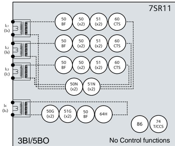
Fig 2. Four Pole Overcurrent Relay Version A software
