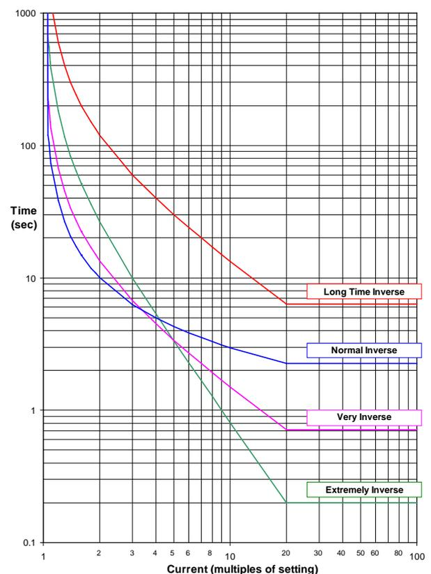
Fig 6. IEC Overcurrent Curves
