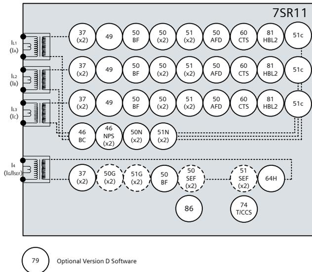
Fig 3 Four Pole Overcurrent Relay Version C Software
